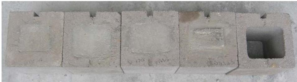
**Figure 27:** Impact-echo specimens from left to right: solid, one small void, many small voids, one large void, and empty
