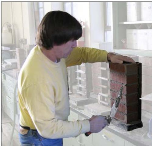
**Figure 9:** Masonry prism construction.
